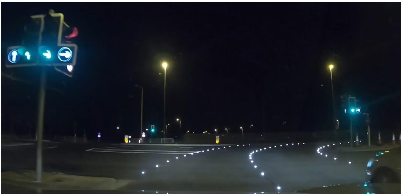
Figure 6-10: An example of illuminated studs from Clearview Intelligence
